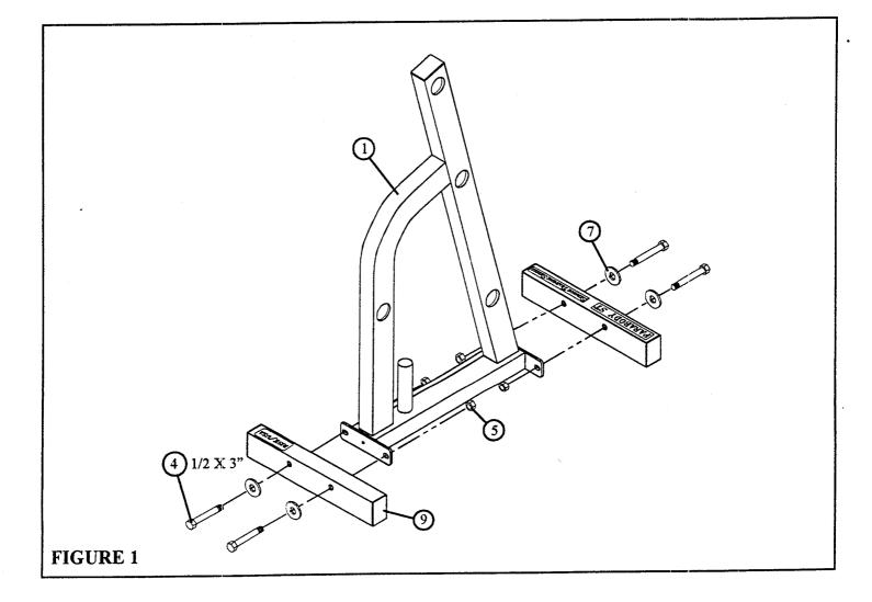
STEP 1: SECURELY assemble two 3 X 2 X 18" TUBES (9) to the FRAME WELDMT (1) using four 1/2 X 3" BOLTS (4) four 1/2" FLAT WASHERS (7) and four 1/2" LOCKNUTS (5) as shown in FIGURE 1.
